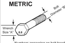
Numbers appearing on bolt heads indicate ASTM class.
